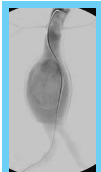
Figure 3. Angiographic image of one of the replicas, perfused with contrast agent, in the flow rig
