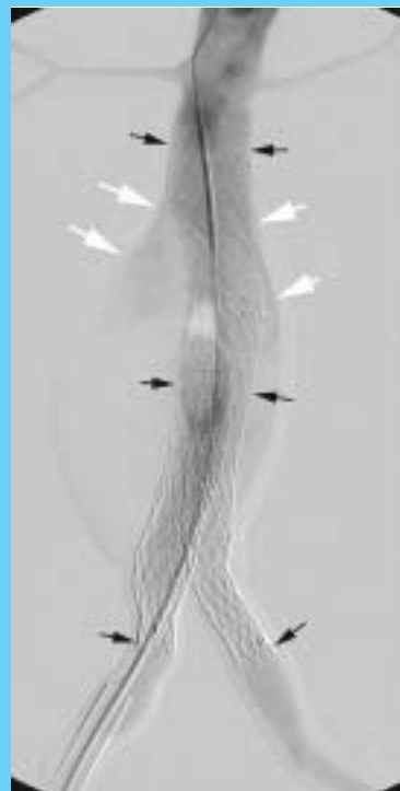
Figure 3. Angiographic image of one of the replicas, perfused with contrast agent, in the flow rig
