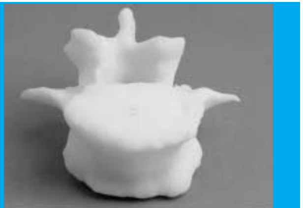
Figure 2. Individual vertebra made of epoxy resin and bone analogue grade hydroxylapatite
