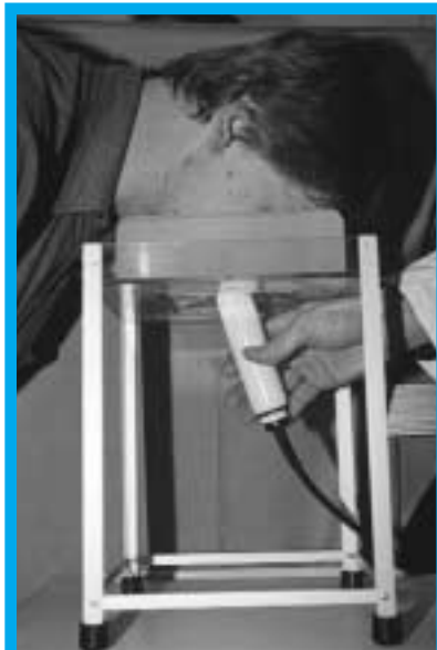
Fig. 1: Water bath with liquid medium based on silicone
