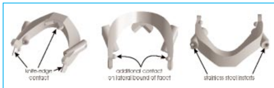
Figure 1: General features of the final drill guide concept for lumbar spine applications.
